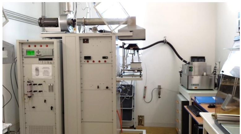
Figure 12. Cone calorimeter (FTT, UK)
